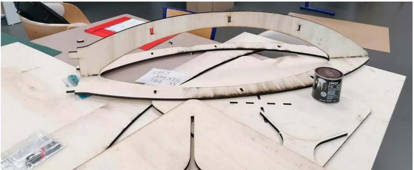
This part is little bit tricky if you are using laser and your material is not completely flat or your laser not well calibrated. The consequences is that laser will not have correct focus on different places on the board. This was my problem and what I did was to divide the drawing into multiple parts and cut each of them separately while adjusting the focus for every color. (see drawing below)
