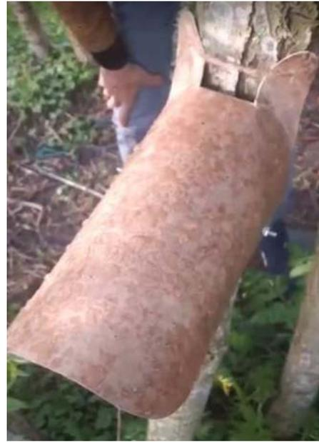
Figure 7: Samples infused with beeswax are tested outside.
